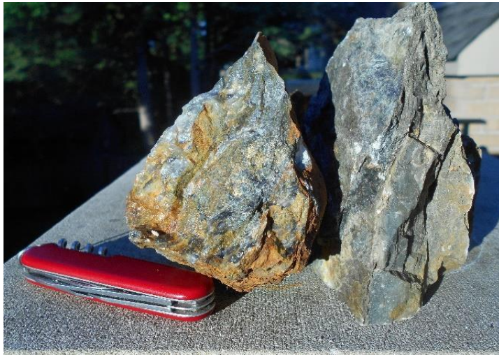
Sheared porphyry with sulphide mineralized quartz veins from Cole mine dump
