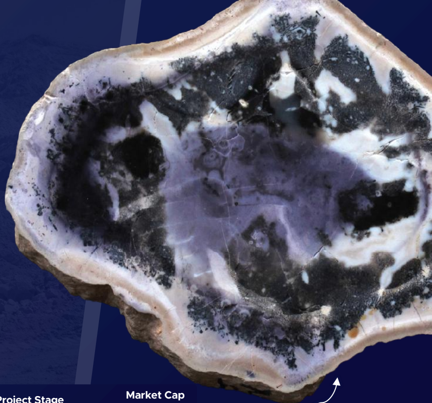
Sample of large layered nodule from the Materion roadside pit showing fluorite, opal, and bertrandite mineralization.
